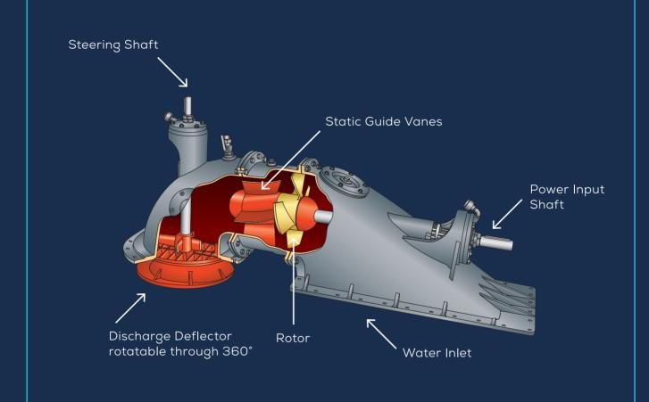
A completely self-contained unit, our horizontal shaft unit, HJP, requires no additional seachest, allowing for a simple installation.
